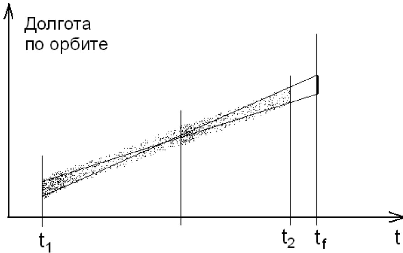
$$\sigma_{\lambda(t_f)} = \sigma_{\dot{\lambda}} (t_f - t_2) = \frac{\sigma_{\lambda}}{t_2 - t_1} (t_f - t_2).$$
